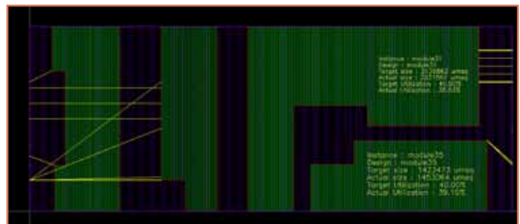
UniPlan provides rapid feedback after block placement for rectilinear blocks with area and utilization.
