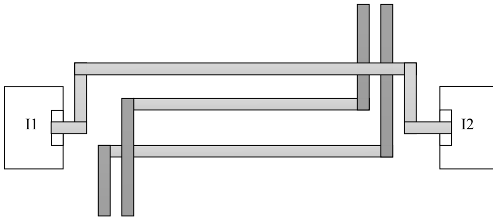
Figure 4: Illustration of the effects of finding alternative path (parasitic constraint driven routing)
